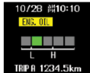
The new dash has a colour display that shows important information such as average and current fuel consumption, oil level and service replacement requirements.
