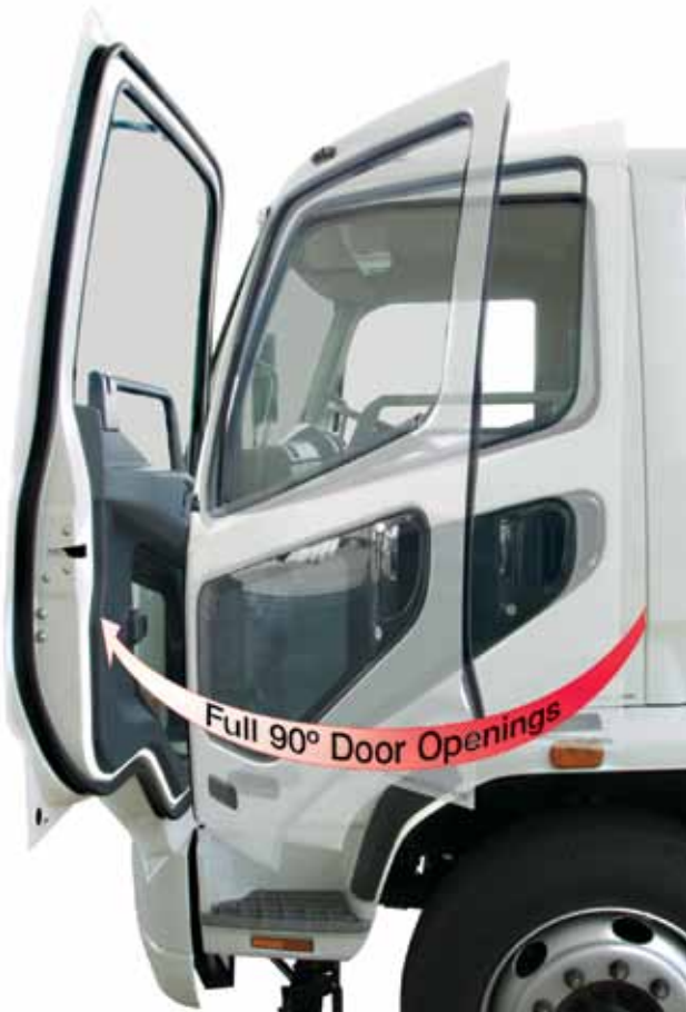
Full 90 degree door opening for easy access. Passenger door has a transom window for improved visibility.
