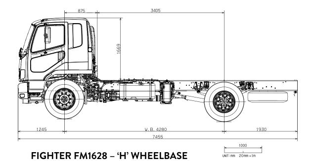
Scale = 1:50 (20mm = 1 metre). This scale is accurate when used on the original spec sheet, be aware that enlarging these illustrations can alter the scale and cause incorrect measurements. Fuso New Zealand and its authorised dealers always recommend customers seek professional advice from independent sources before commencing any engineering activities.
