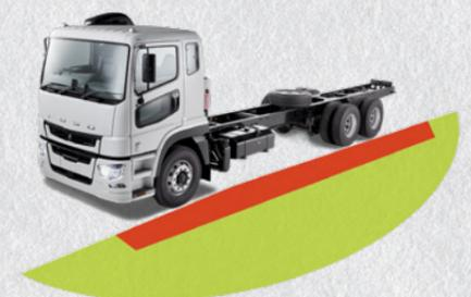
ASGA detects moving objects on the left-hand side of the vehicle, triggering an eye-level warning light to attract the driver's attention to the left-side wing mirrors. If there is a risk of collision, the warning light flashes several times in red. After two seconds, it remains permanently illuminated in red and, in the event of an imminent collision, a warning tone also sounds.
