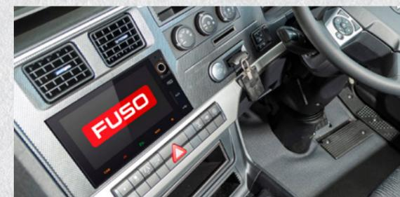
Steering wheel controls enable safe operation. An on-dash screen relays images from a high-definition, infrared reversing camera. The system works with Apple CarPlay and Android Auto for hands-free talking and text-to-speech functionality. It also works with other handy apps such as Google Maps and Spotify.
